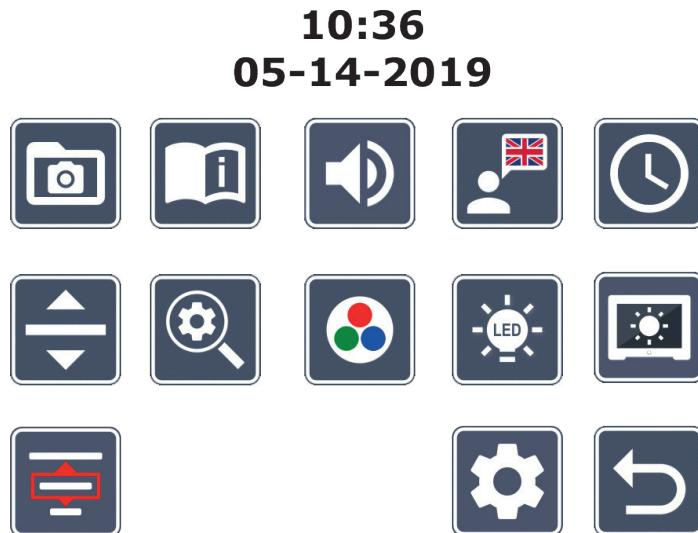
You can move to the individual symbols using the rotary knobs ② + ⑧ and the arrow keys ⑫, ⑬, ⑯, ⑰. The symbol for the selected function becomes larger and is displayed in colour. Press the button ③ to activate each selected function.
